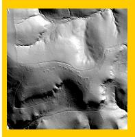
May's image: LiDAR (Light Detection And Ranging) is an aircraft based tool that uses radar energy to image the ground surface through trees and other vegetation. It is capable of imaging surface relief of a few inches or less. Iowa was one of
