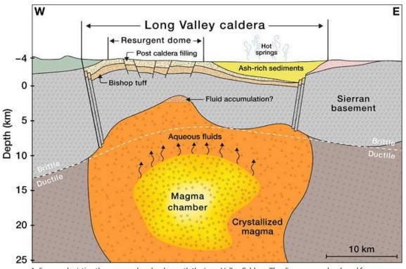
A diagram depicting the magma chamber beneath the Long Valley Caldera. The diagram was developed from tomographic imaging using seismic waves.
